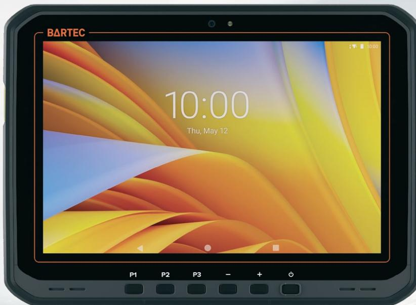
**The BARTEC ET60/65 Ex2 delivers powerful mobile computing for Zone 2 environments in a slim, rugged design.**
